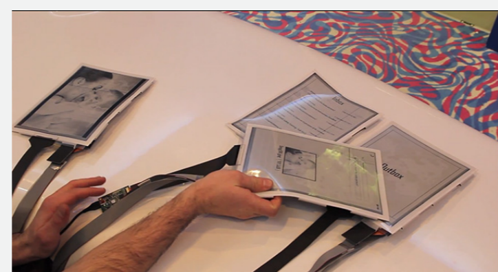
Fig. 3 Papertab . Flexible e-ink touchscreen display (accessed at extremetech.com).
