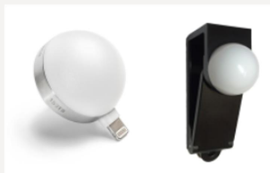
Figure 2 – External light sensors.
